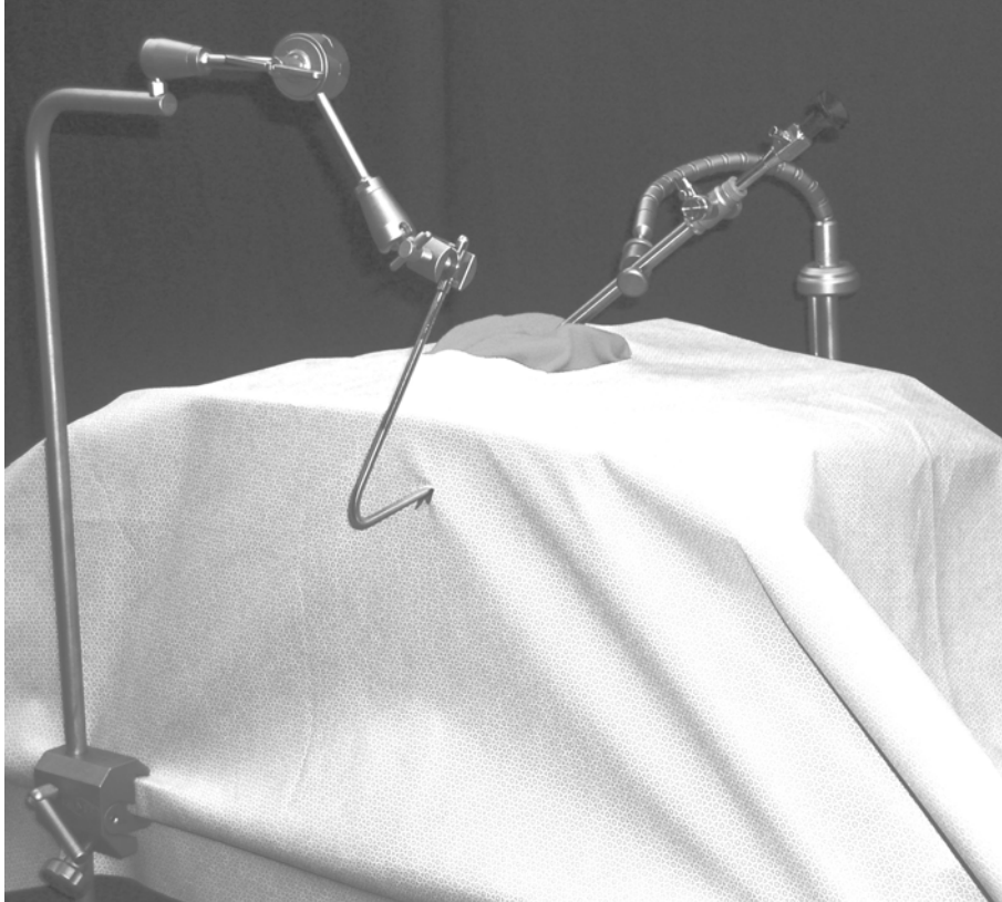
Retract-Robot holding a Nathanson Liver Retractor & Goose Neck Retractor holding Laparoscope
